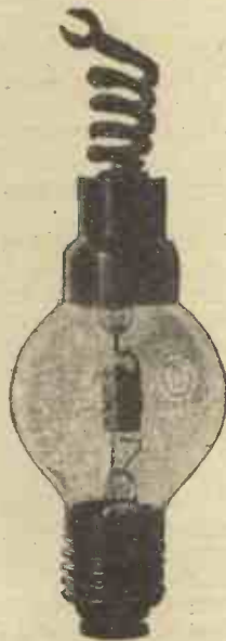
Fig. 1. A two-electrode valve for rectification of H.T. supply.
