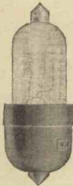
Fig 1. A specially designed valve for short wave work: the Mullard "Ora B."
