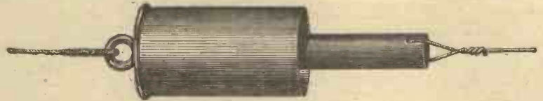
Fig. 11. The completed insulator.
